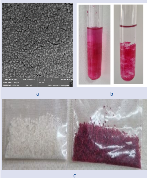
Figure 4. (a) SEM images of the hydrogels, (b) photos of carminic acid solution before/after adsorption, (c) photos of dried the hydrogels before/after adsorption.
