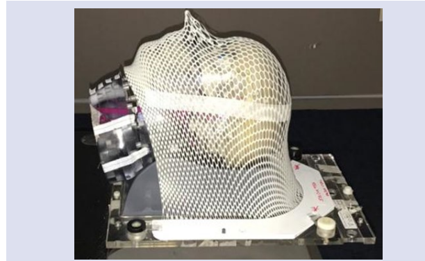
Figure 1. Fixing the phantom with a thermoplastic mask. Picture is taken during the measurements in the laboratory of Medicana Ankara hospital.
