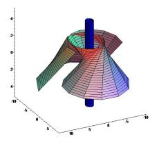
FIGURE 2. Cylinder (colored with blue) and the involute offset of the cylinder with  $\phi^* = 45^{\circ}$  and  $\psi = 45^{\circ}$
