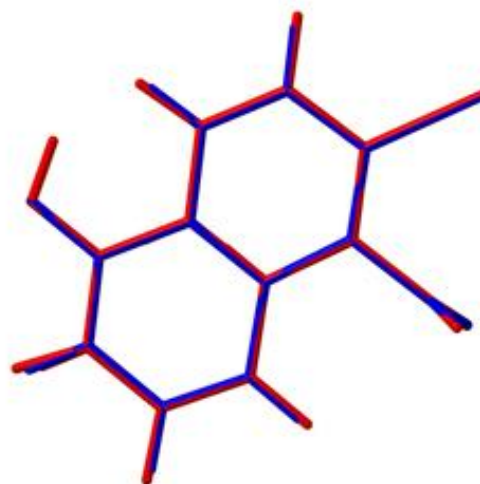
Figure 4. Atom-atom superposition of (red) structure calculated on X-ray structure (blue) for compound 3 .
