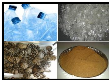
Figure 1. Organic reinforcement for polyester composite; Pine cones and PET bottle chips.
