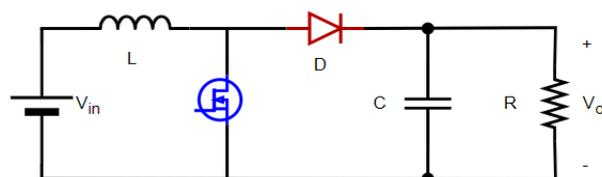
Figure 4. Boost converter circuit topology
