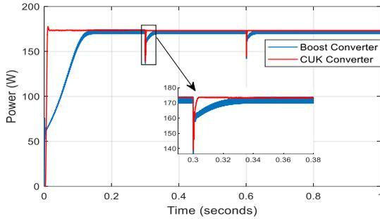
**Figure 16.** Boost converter and CUK converter output powers
