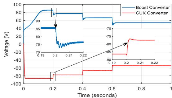
Figure 12. Boost converter and CUK converter output voltages
