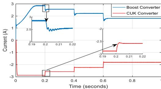
Figure 11. Boost converter and CUK converter output currents
