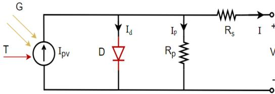
Figure 1. Single diode PV cell model [16]
