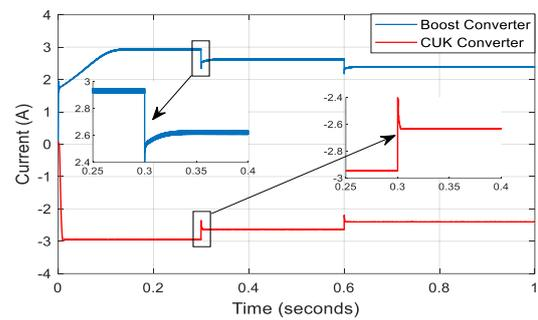
Figure 14. Boost converter and CUK converter output currents
