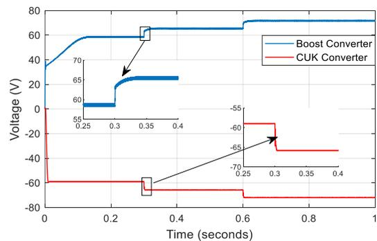
Figure 15. Boost converter and CUK converter output voltages
