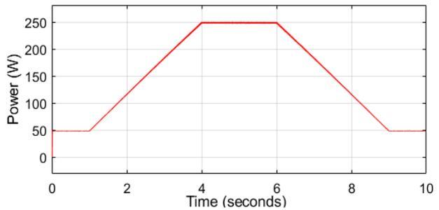
**Figure 18.** Boost converter output power
