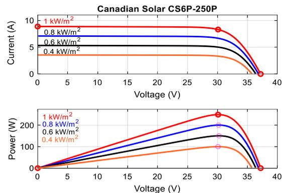
Figure 3. PV system curves at fixed 25°C temperature value
