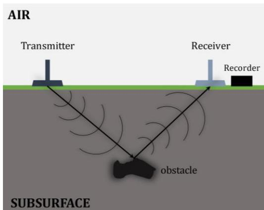
**Figure 6.** Schematic demonstration of the working principle of a typical GPR system
