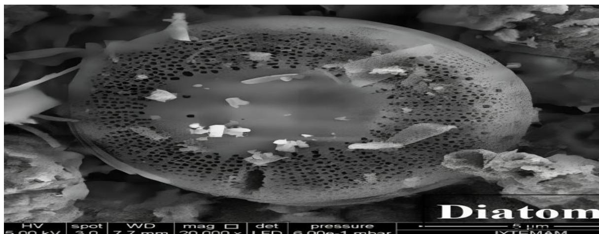
Figure 1. Scanning electron microscope image of Almina DE
