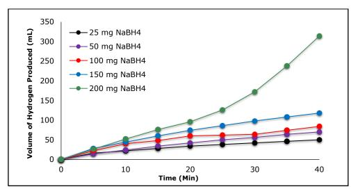
Figure 7: Effect on hydrogen volume of NaBH<sub>4</sub> using Fe<sub>3</sub>O<sub>4</sub>@SA MNCs (Reaction conditions: 50 mg nanocatalyst, 25, 50, 100, 150 and 200 mg NaBH<sub>4</sub> and 25 °C).
