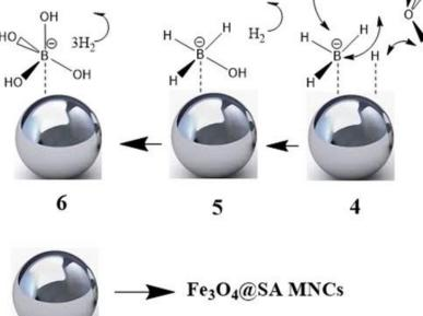
**Figure 10:** A possible mechanism of NaBH<sub>4</sub> hydrolysis catalyzed by Fe<sub>3</sub>O<sub>4</sub>@SA MNCs.
