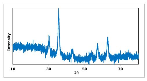
Figure 3: Fe<sub>3</sub>O<sub>4</sub>@SA MNCs XRD pattern.
