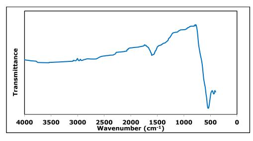
Figure 2. Fe<sub>3</sub>O<sub>4</sub>@SA MNCs FTIR spectrum.
