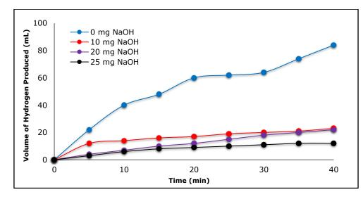
**Figure 6:** Effect on hydrogen volume in NaBH<sub>4</sub> hydrolysis of NaOH (Reaction conditions: 50 mg Fe<sub>3</sub>O<sub>4</sub>@SA MNCs, 100 mg NaBH<sub>4</sub>, 0, 10, 20 and 25 mg NaOH and 25 °C).
