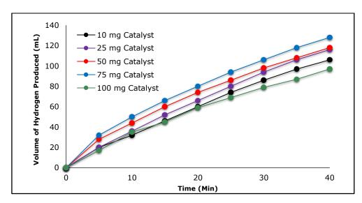
**Figure 8:** Effect on hydrogen volume by hydrolysis of NaBH4 of Fe<sub>3</sub>O<sub>4</sub>@SA MNCs (Reaction conditions: 10, 25, 50, 75, and 100 mg Fe<sub>3</sub>O<sub>4</sub>@SA MNCs, 150 mg NaBH<sub>4</sub> and 25 °C).
