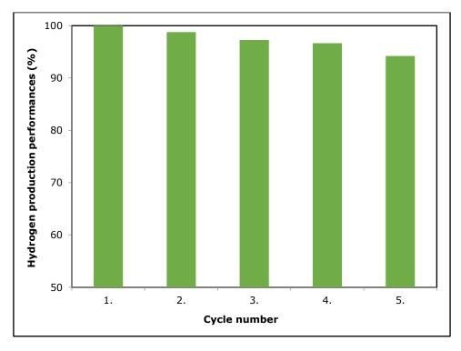
Figure 9: The reusability of Fe<sub>3</sub>O<sub>4</sub>@SA MNCs for hydrolysis of NaBH<sub>4</sub> at 25 °C.
