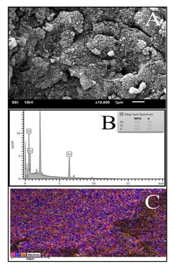
**Figure 5:** Fe<sub>3</sub>O<sub>4</sub>@SA MNCs A) SEM images, B) SEM-EDS graph, C) SEM-EDS-map graph.
