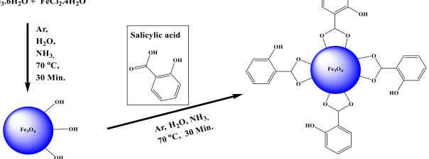
Figure 1. The synthesis scheme of Fe<sub>3</sub>O<sub>4</sub>@SA MNCs.
