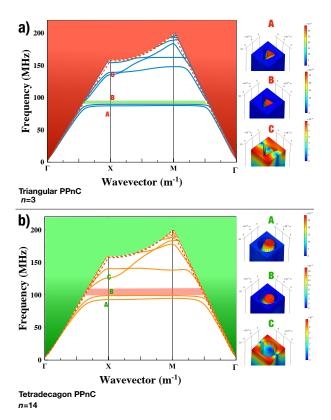
**Figure 2.** Band profile of a) triangular (n=3) cavity type and b) tetradecagon (n=14) type PPnC and corresponding displacements in the resonance frequencies.
