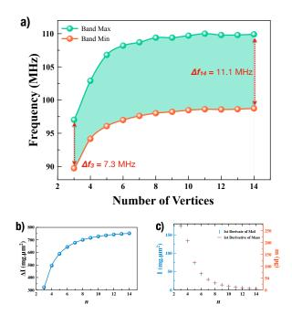
**Figure 4.** a) Changes in the frequencies at the edges of the LRBG with respect to the number of vertices of polygonal cavity-type PPnC, b) the moment of inertia difference ( $\Delta I$ ) of groove and pillar as a function of the number of vertices that equals to the extracted part to create the cavity and c) 1st derivatives of the moment of inertia and mass of the extracted part of the polygonal cavity-type PPnC.
