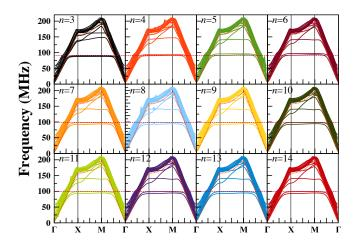
Figure 3. The band structures of the square array polygonal cavity-type PPnCs for the different number of vertices.
