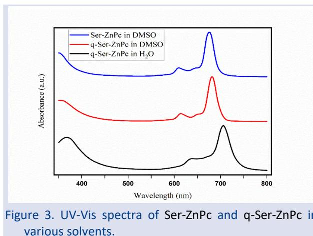
Figure 3. UV-Vis spectra of Ser-ZnPc and q-Ser-ZnPc in various solvents.
