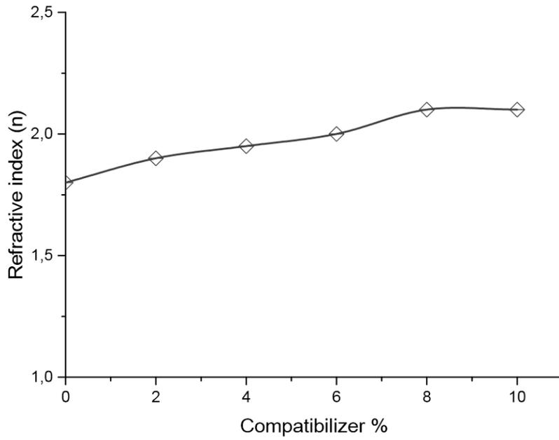
Figure 5. Relation of refractive index MASTMMA compatibilizer ratio
