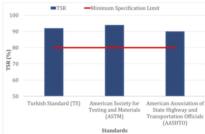
Figure 12. Tensile strength ratios of samples
