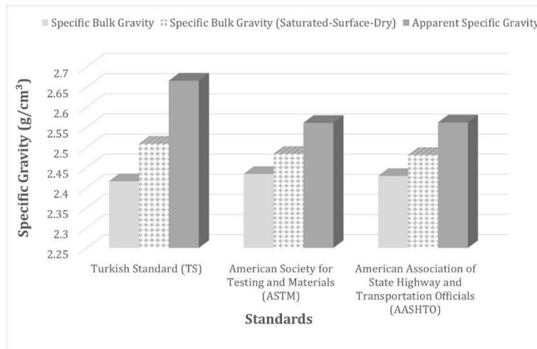
**Figure 5.** Specific gravity values of fine aggregates
