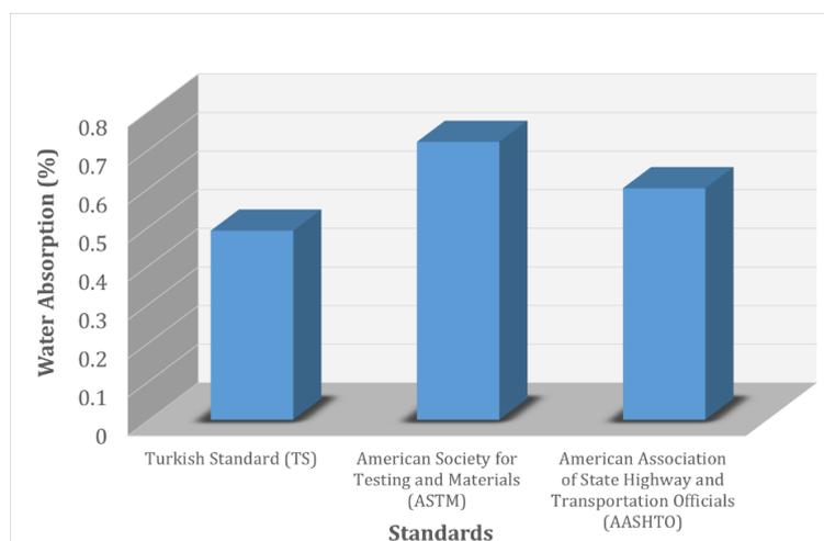
**Figure 4.** Values of water absorption of coarse aggregates
