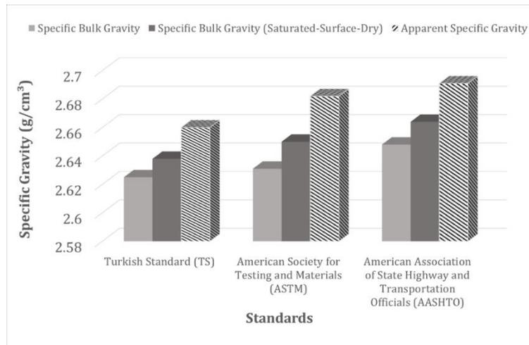
**Figure 3.** Specific gravity values of coarse aggregates
