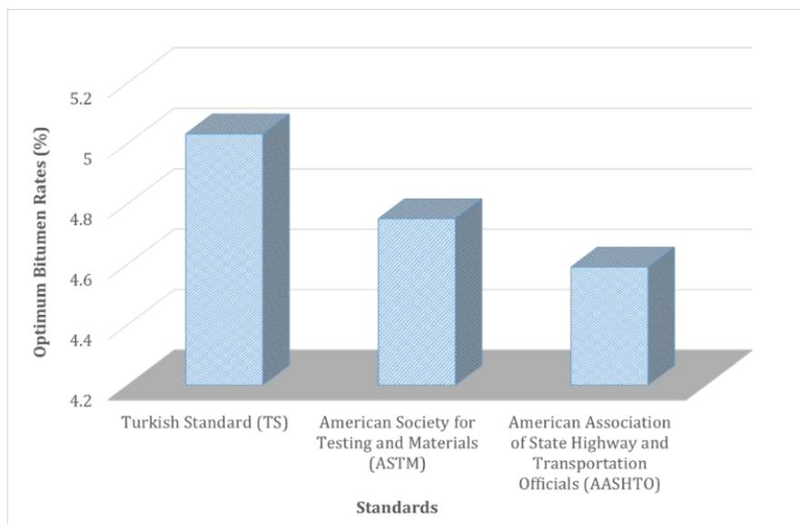
Figure 10. Optimum bitumen contents according to standards
