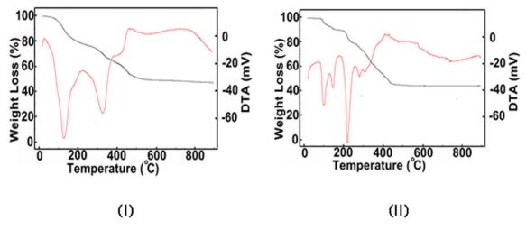
Figure 3. TGA/DTA curves of histidine (I) and arginine (II) pentaborate structure.
