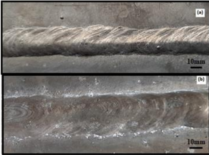
Figure 2. Images of plate samples joined by (a) MIG welding (b) TIG welding
