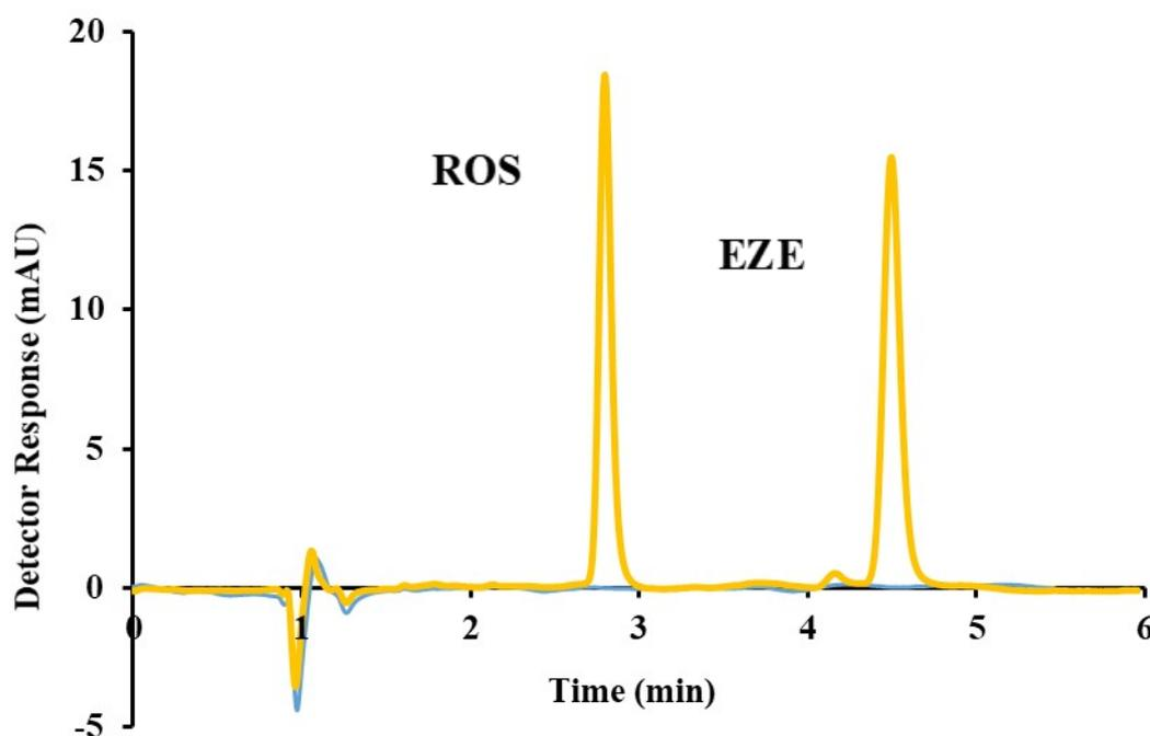
**Figure 3:** The chromatogram of 5 µg/mL Rosuvastatin and Ezetimibe from prepared tablet formulation.
