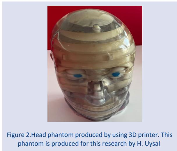
Figure 2. Head phantom produced by using 3D printer. This phantom is produced for this research by H. Uysal
