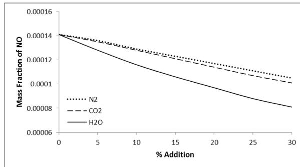
**Figure 6.** The mass fractions of NO at different N<sub>2</sub>, CO<sub>2</sub>, and H<sub>2</sub>O addition rates.
