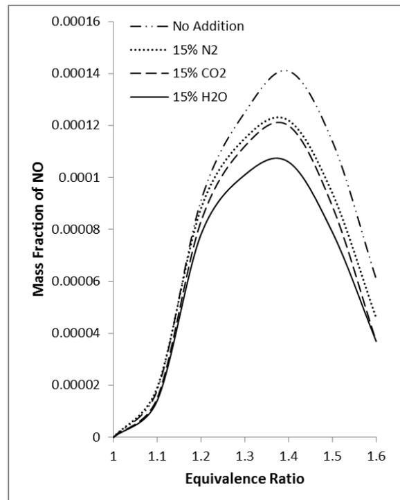
**Figure 5.** The mass fractions of NO at different equivalence ratios.
