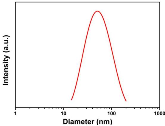
Figure 1. Particular size analysis of synthesized Hap powders
