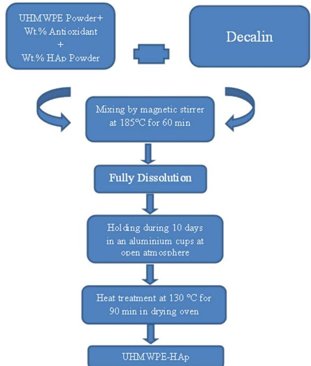
Figure 2. Schematic illustration of UHMWPE-HAp composites preparation.
