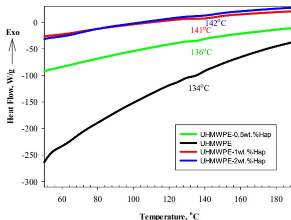
Figure 7. DSC analysis of the UHMWPE and UHMWPE HAp composites.
