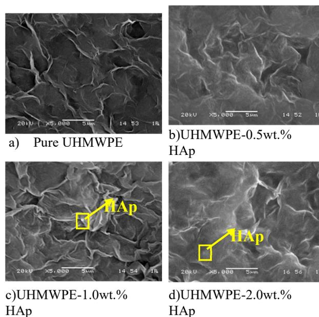
Figure 4. SEM surface images of a) pure UHMWPE, b) UHMWPE- 0.5wt.%HAp, c) UHMWPE- 1 wt.%HAp and d) UHMWPE- 2 wt.%HAp.
