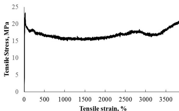
Figure 8. Tensile test curve of UHMWPE-1wt.%HAp.
