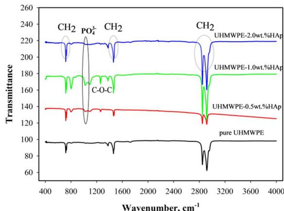
Figure 6. FT-IR spectra of UHMWPE and UHMWPE-0.5wt.%HAp, 1wt.% HAp and 2wt.% HAp composites.
