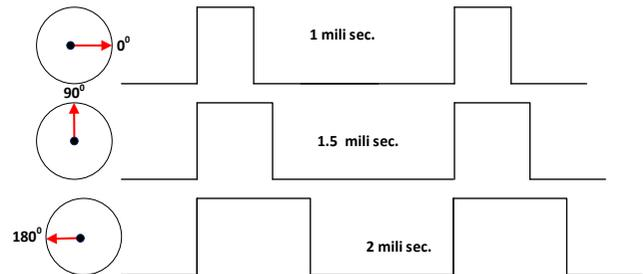
Figure 2. Shaft angle values and PWM signals.
