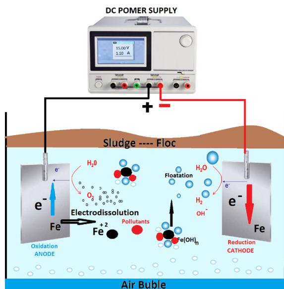
**Figure 1.** Schematic presentation of air-assisted electrocoagulation process.
