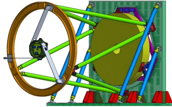
Figure 4. Cassegrain collimator mechanical assembly.
