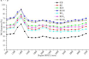
Figure 10.NO Emission Change Depending on the Engine Speed
