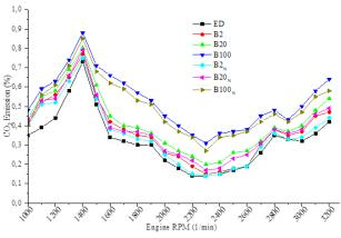
Figure 8.CO<sub>2</sub> Emission Change Depending on the Engine Speed
