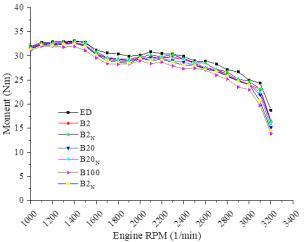
Figure 2. Change of the Torque Values of ED, Biodiesel and Fuel Blends Depending on the Engine Speed
