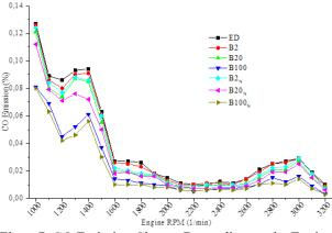
Figure7. CO Emission Change Depending on the Engine Speed
