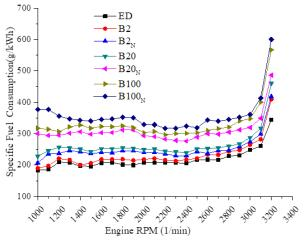
Figure 4. Specific Fuel Consumption Value Change Depending on the Engine Speed When ED, Biodiesel and Fuel Blends were Used
