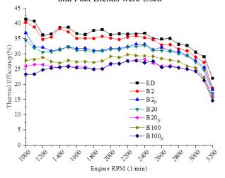
Figure 5. Thermal Efficiency Value Changes Depending on the Engine Speed of ED, Biodiesel and Fuel Blends
