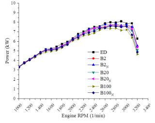
Figure 3. The Power Change Depending on the Engine Speed when Biodiesel, ED and Fuel Blends were Used The changes of specific fuel consumption, one of the engine properties, depending on the engine speed are shown in Figure 4. There was 47.11% increase in specific fuel consumption when WCOB fuel was used at maximum power (2900 1/min) in comparison to ED, and there was 52.05% increase when NWCOB fuel was used in comparison to ED. As a result of the tests
