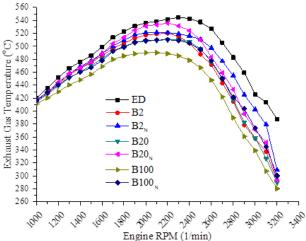
Figure 6. The Exhaust Gas Temperature Value Changes Depending of the Engine Speed of ED, Biodiesel and Fuel Blends
