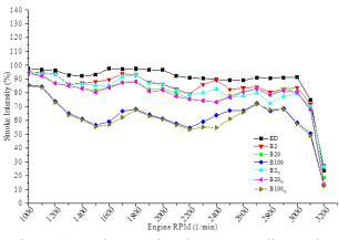
Figure 11. Smoke Intensity Change Depending on the Engine Speed
