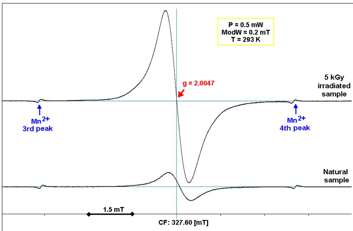
**Figure 2.** ESR spectra of natural and 5 kGy irradiated coffee bean samples.
