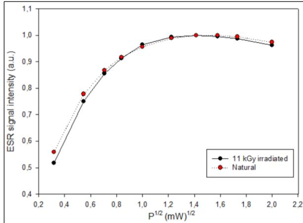
Figure 3. Microwave dependence of  $g=2.0047$  signal.
