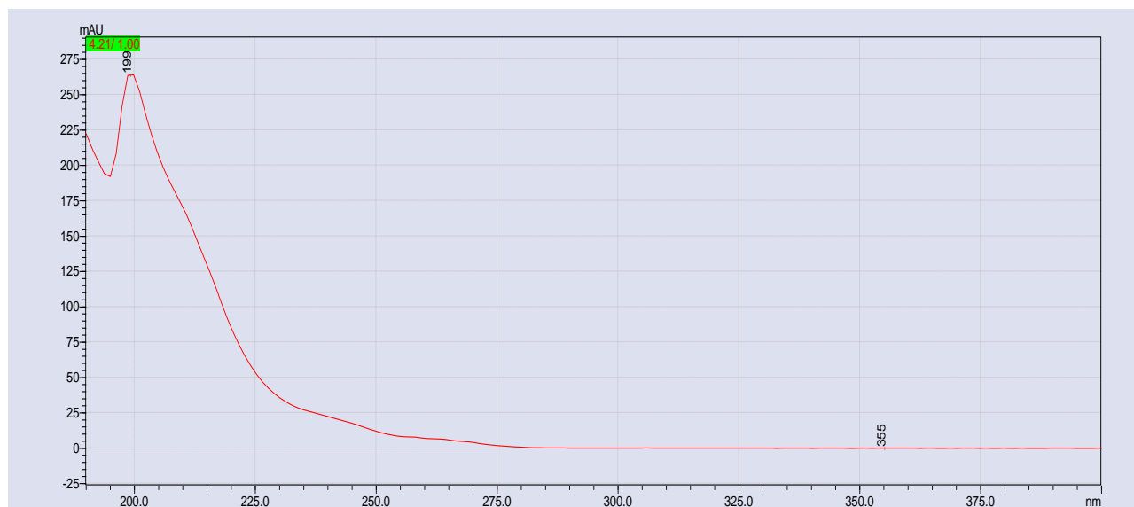
Figure 4. UV-VIS Spectrum obtained in DAD Detector for Phenobarbital
