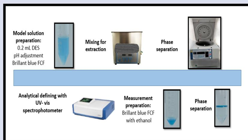
Figure 1. Schematic depiction of the DB-DLLME technique
