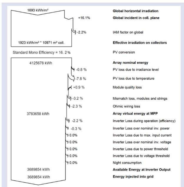
Figure 9. Standard Mono Cell losses and efficiency results.
