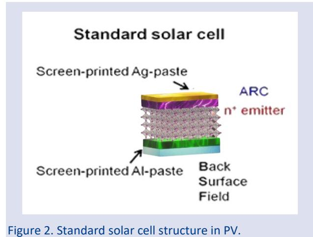
Figure 2. Standard solar cell structure in PV.
