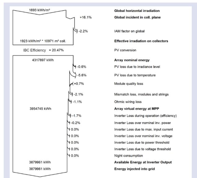
Figure 10. Mono IBC Cell losses and efficiency results.
