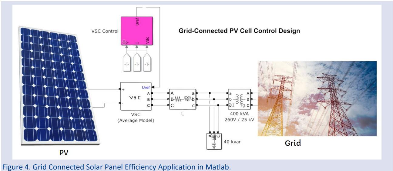
Figure 4. Grid Connected Solar Panel Efficiency Application in Matlab.
