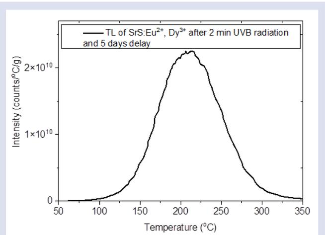
Figure 8. TL Glow curve of SrS: Eu<sup>2+</sup>, Dy<sup>3+</sup> phosphor after 5 days storing at dark atmosphere.
