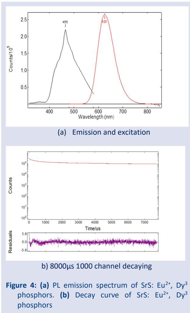
The SrS: Eu<sup>2+</sup>, Dy<sup>3+</sup> phosphors' excitation-emission bands and the PL decay curves at room temperature are shown in Figure 4. The excitation spectrum of emission has a wide band (400- 600 nm) making a peak around 466 nm, corresponding to the host lattice transition. The electromagnetic spectrum's visible area contains the excitation range (Figure 4(a)). When excited, the emission peak appears at 550 nm giving broadband that lasts until
