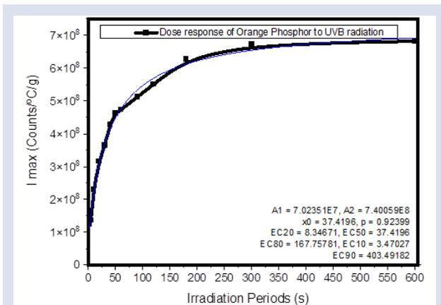
Figure 7. Dose-response curve of SrS: Eu<sup>2+</sup>, Dy<sup>3+</sup> phosphor to UVB radiation
