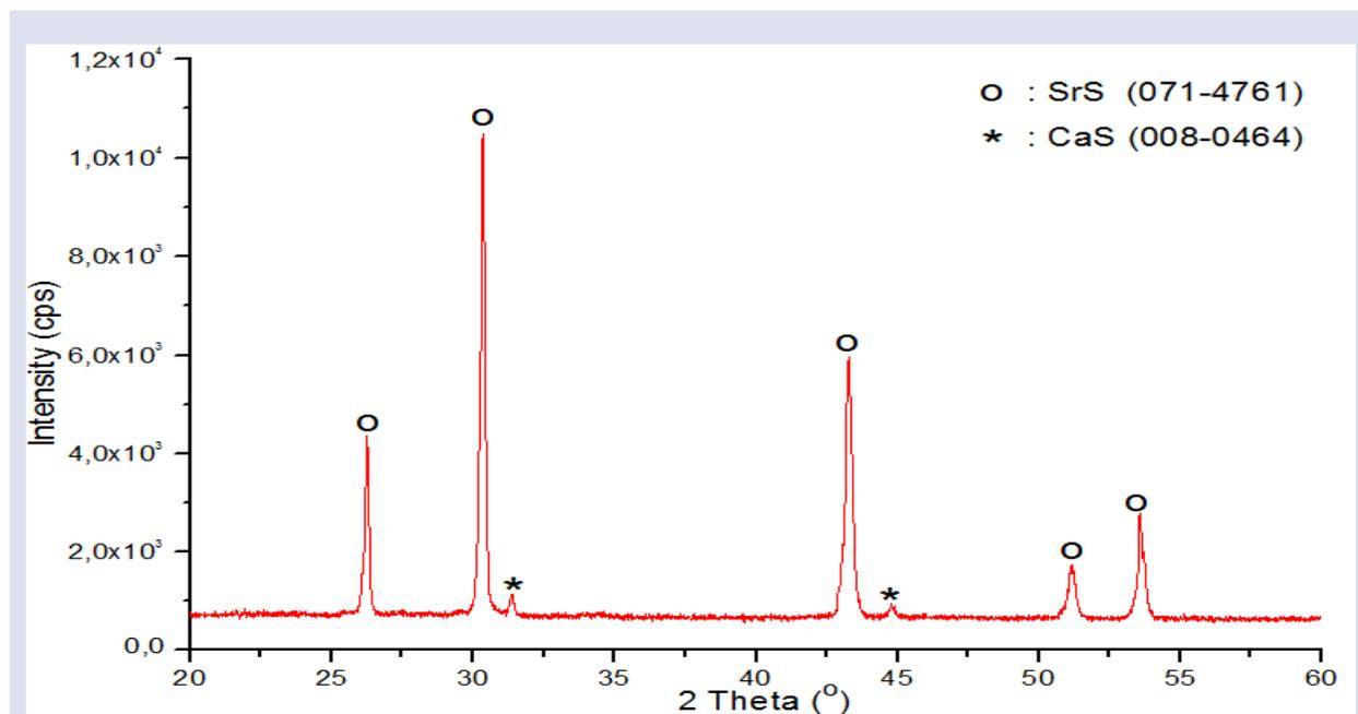
Figure 1. XRD pattern of SrS: Eu<sup>2+</sup>, Dy<sup>3+</sup> phosphor.
