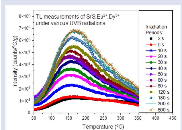
Figure 6. TL glow curves of SrS: Eu<sup>2+</sup>, Dy<sup>3+</sup> phosphor immediately after exposure to various UVB radiation.
