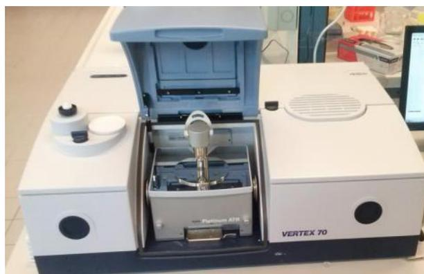
Figure 1. FTIR Spectroscopy Device
