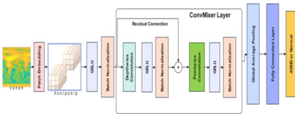
Figure 4. ConvMixer Network Architecture
