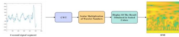
Figure 2. Stages of obtaining HMI
