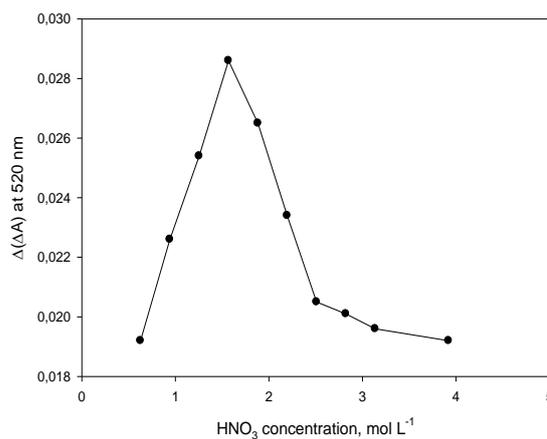
**Figure 2.** Effect of  $\text{HNO}_3$  concentrations on the analytical signal.
