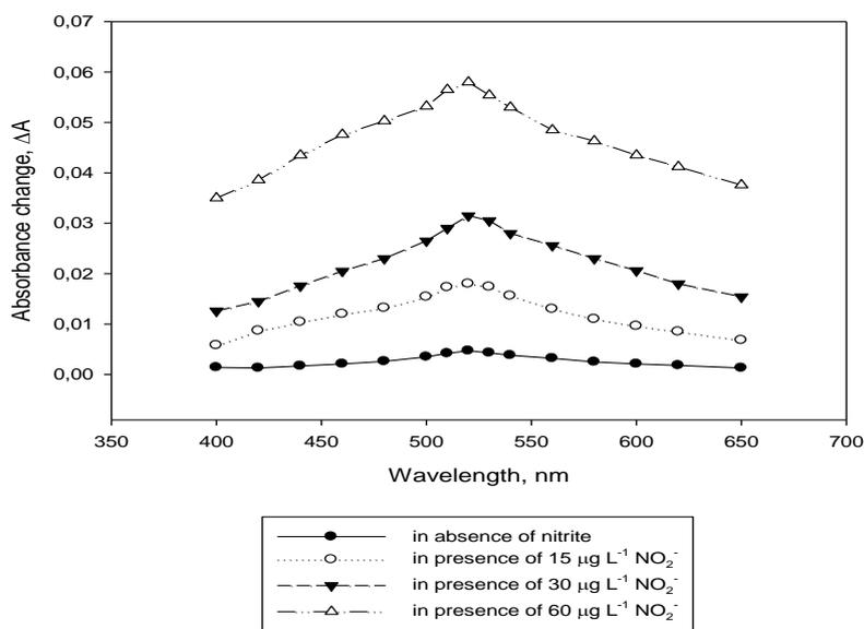
**Figure 1.** Absorbance change of micellar catalyzed indicator system with increasing nitrite concentration as a function of wavelength in presence of 15, 30 and 60  $\mu\text{g L}^{-1}$   $\text{NO}_2^-$ .
