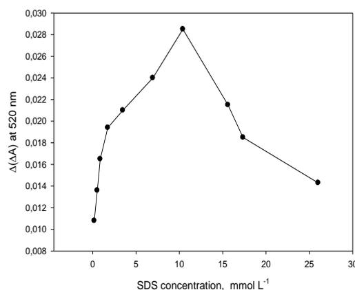
**Figure 4.** Effect of SDS concentration on the analytical signal.
