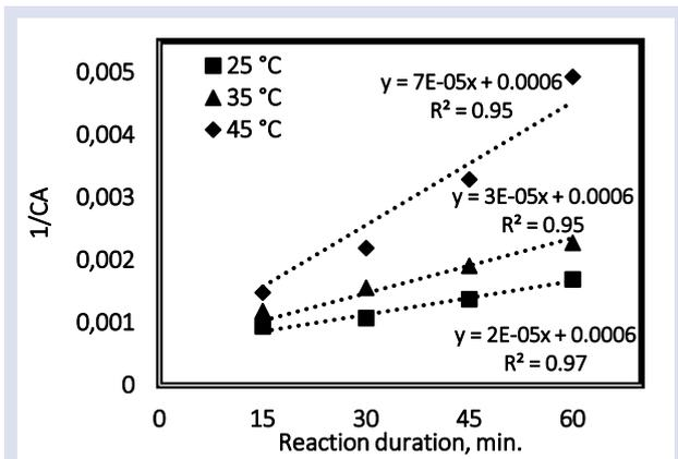
Figure 6. Linearized second-order kinetic plot (Reaction conditions: 100 mL sugar industry wastewater, pH: 3.5, ZVI: 2 g/L, [H<sub>2</sub>O<sub>2</sub>]<sub>0</sub>: 4 mM, T: 25-45 °C t: 60 min)
