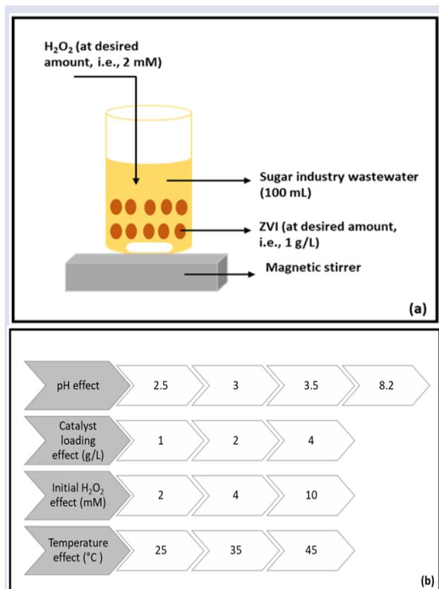
Figure 1. Experimental set-up (a) and reaction conditions (b)
