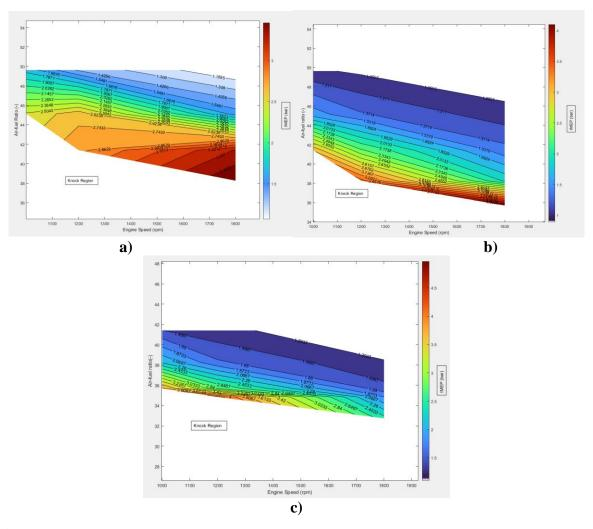
**Figure 10.** Compression ratio effect on HCCI operating range and IMEP (Tin=20°C Pin=0.95 bar) a) 17.5 b) 15 c) 13
