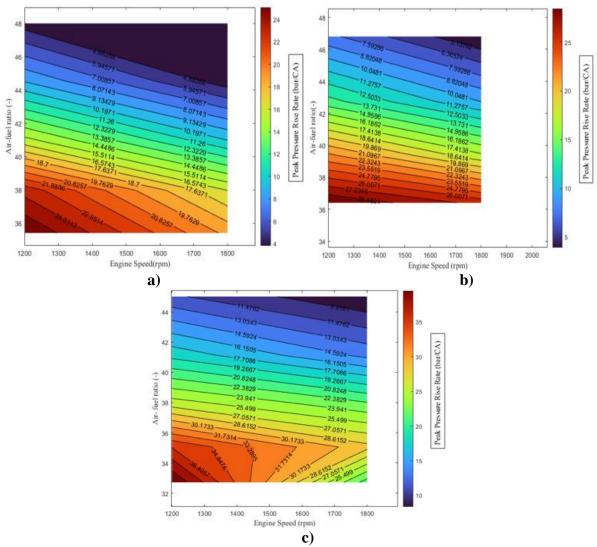
**Figure 11.** Inlet air temperature effect on HCCI operating range and peak pressure rise rate (Pin=0.95 bar CR=17.5) a) Tin=40°C b) Tin=60°C c) 80 °C
