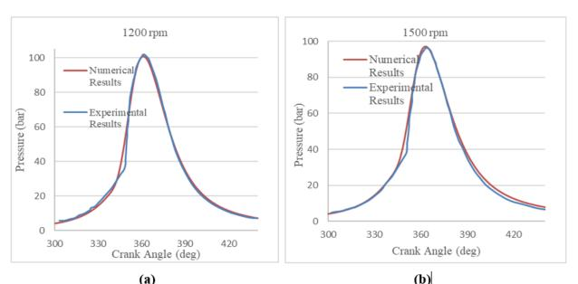
**Figure 6.** In-cylinder pressure at a) 1200 and b) 1500rpm
