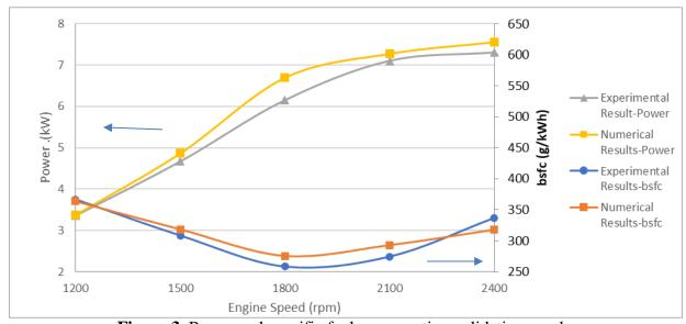
Figure 3. Power and specific fuel consumption validation graphs
