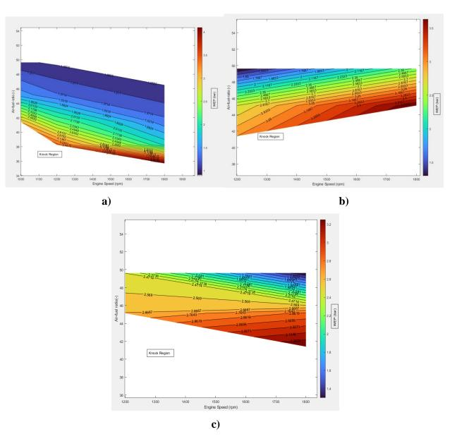
**Figure 13.** Inlet air temperature effect on HCCI operating range and IMEP (Pin=0.95 bar CR=15) a) Tin=20°C b) Tin=40°C c) 60 °C
