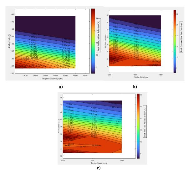
**Figure 12.** Inlet air temperature effect on HCCI operating range and peak pressure rise rate (Pin=0.95 bar CR=15) a) Tin=40°C b) Tin=60°C c) 80 °C
