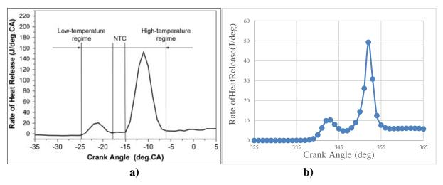
**Figure 8.** Heat Release Curve a) Typical curve for HCCI combustion with n-heptane [28] b) obtained from the model for 1200 rpm, Pin=0.95 bar Tin=20°C, AFR=45
