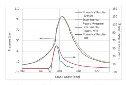
Figure 5. In-cylinder pressure and HRR at 1800 rpm
