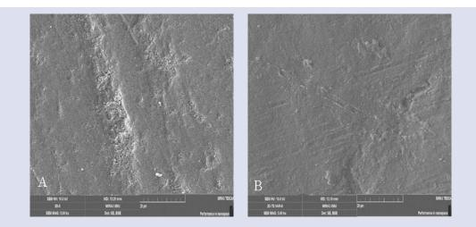
*Figure 5: Image of surface properties of samples obtained by 3D printing at x5000 magnification under SEM. A: Nothermocycling, B: Thermocycling.*
