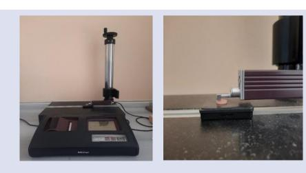
Figure 2: Profilometer device and surface roughness measurement.
