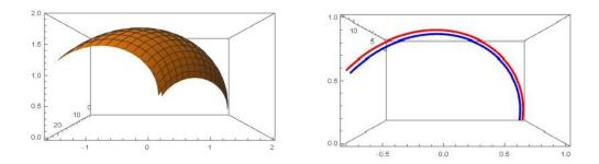
FIGURE 1. Translation surface and its generating curves  $\mathbf{x}(\text{Red})$  and  $\mathbf{y}(\text{Blue})$  for Bertrand partner curve.
