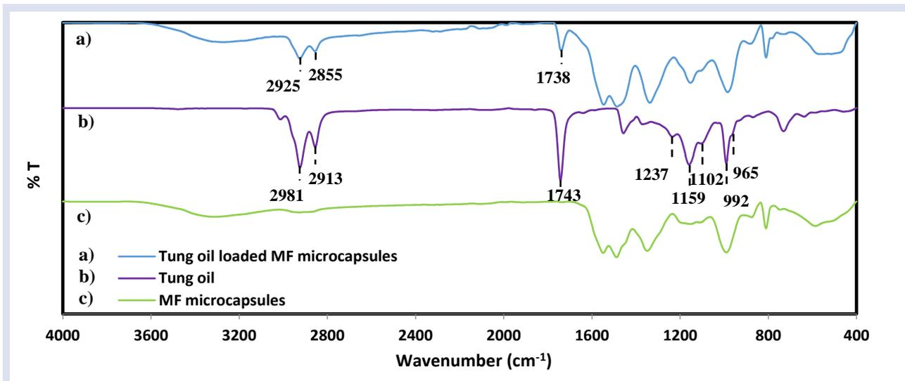
Figure 4. FTIR spectra of a) tung oil loaded MF microcapsules, b) tung oil and c) MF microcapsules.
