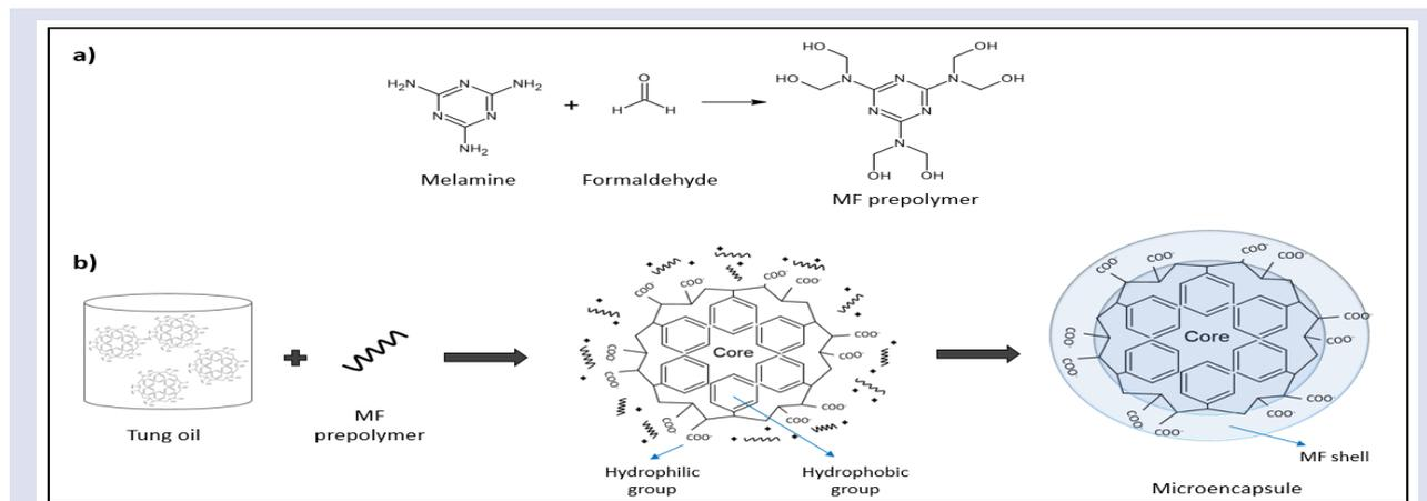
Figure 2. a) MF prepolymer formation mechanism, b) Schematic illustration of the synthesis of microencapsulation of tung oil.
