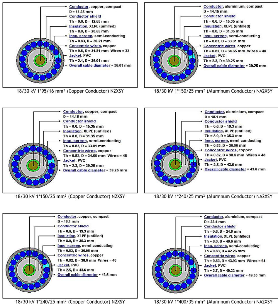
Figure 2. The design of the cables with CYMCAP
