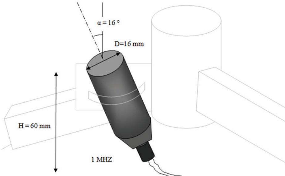
*Figure 2 - Ultrasonic Velocity Profile (UVP) transducer configuration*
