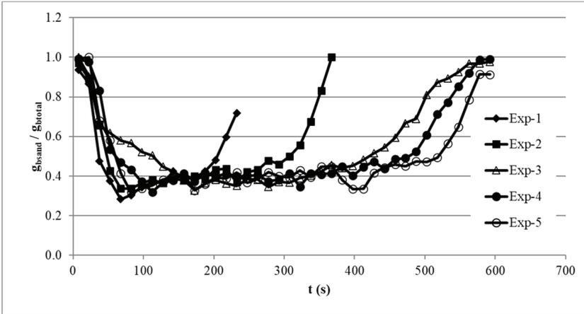
Figure 11 - Time variations of the sand content ratio of the bed load
