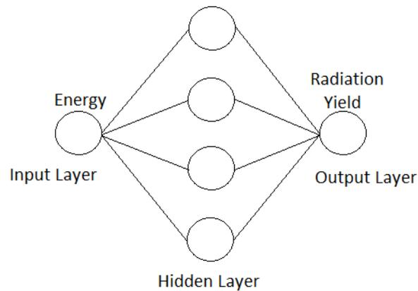
**Fig. 1** ANN architecture of 1-4-1 for estimation of radiation yield for various materials
