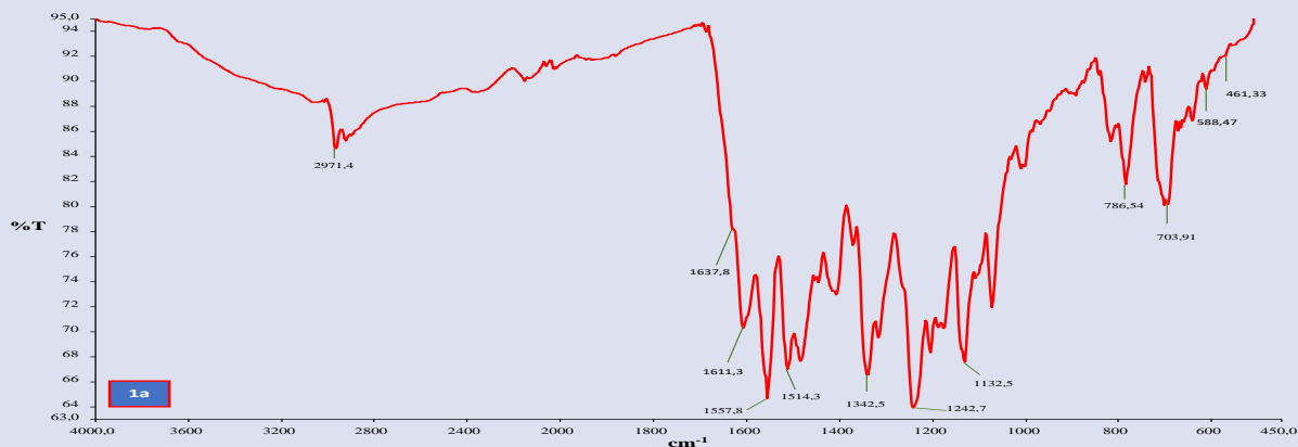
Figure 3 FTIR spectrum of the Co(II) - Ligand complex structure.
