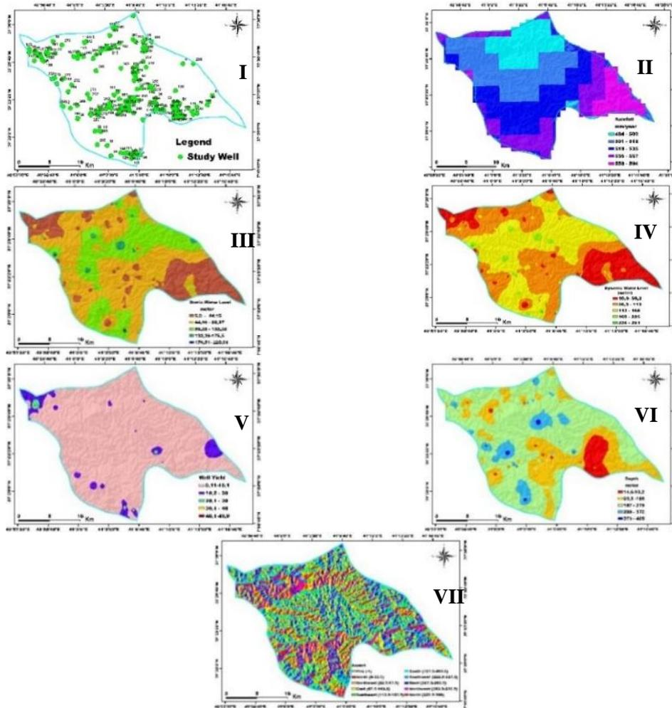
**Figure 3.** Thematic maps created according to the outline of the study (I. Study well, II. Rainfall, III. Static water level, IV. Dynamic water level, V. Well yield, VI. Depth, VII. Aspect map) After the creation of raster thematic maps, these maps were reclassified (Figure 4) [21-27].
