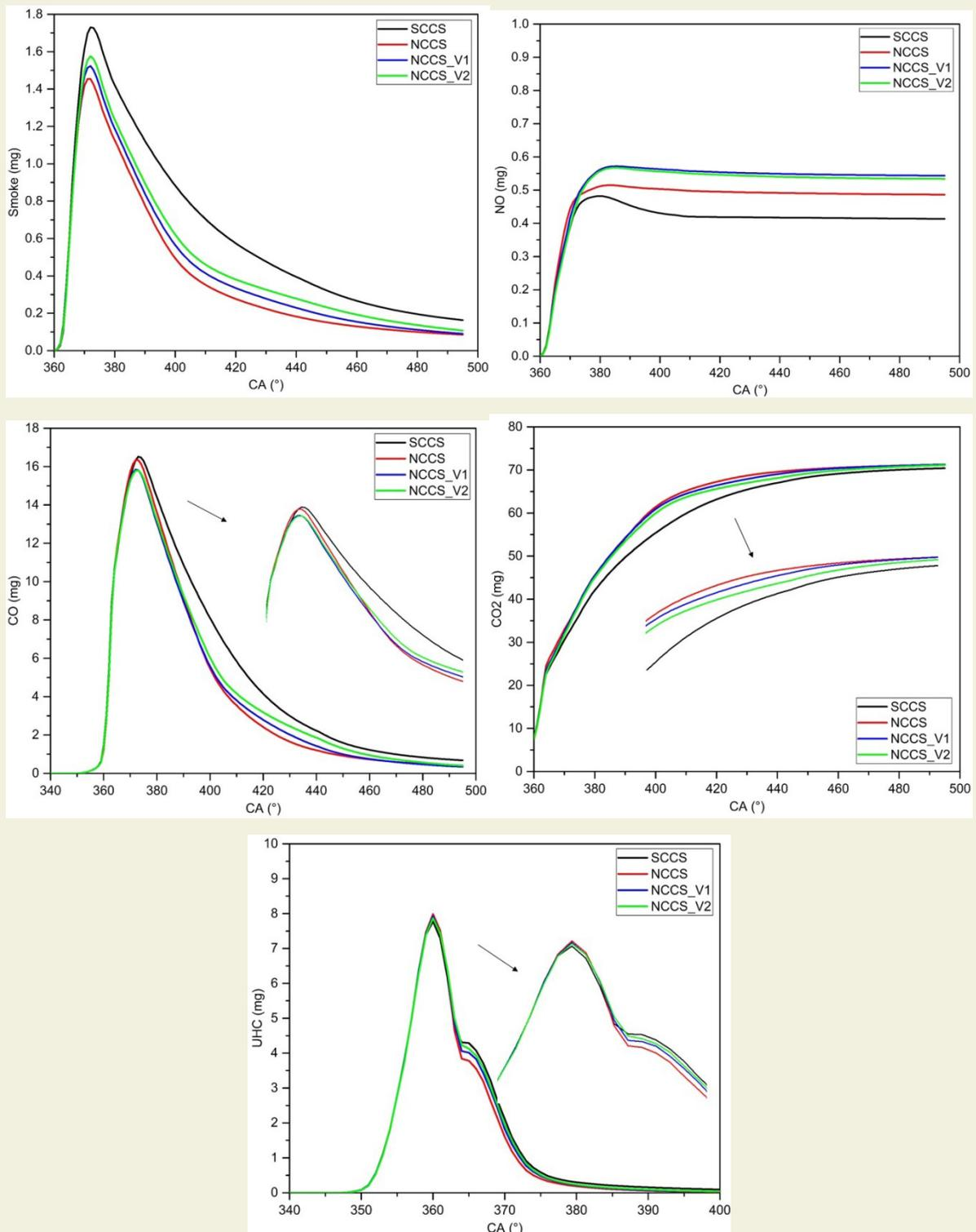
Figure 5. Change of exhaust emission values (Smoke, NO, CO, CO<sub>2</sub> and UHC) obtained for NCCS and SCCS geometries
