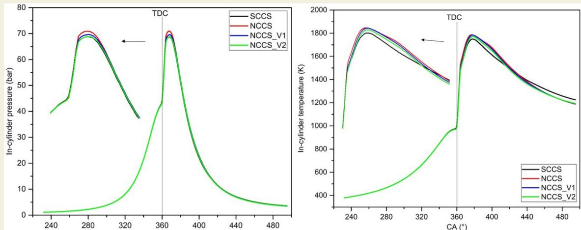
Figure 2. Change of in-cylinder pressure and temperatures with crank angle for NCCS and SCCS geometries
