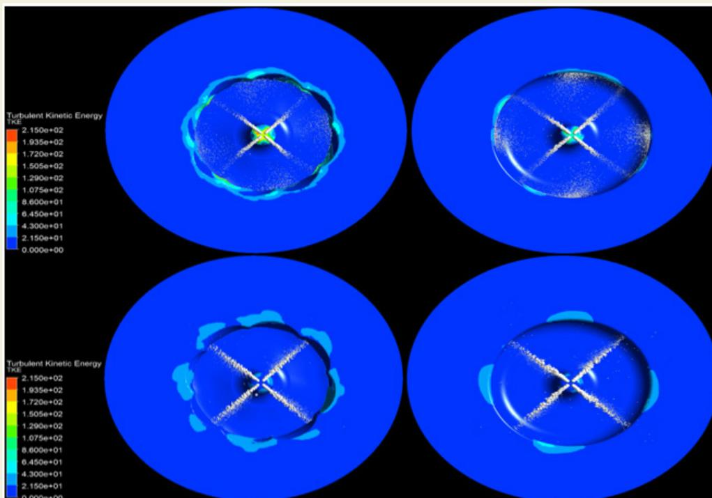
Figure 7. TKE changes of NCCS and SCCS geometries
