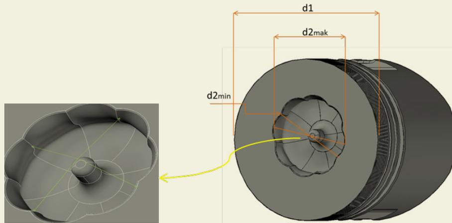
**Figure 1.** Piston bowl and fuel injection direction
