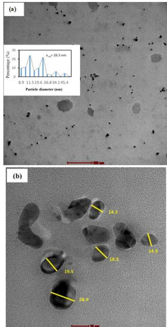
Figure 6. TEM image of spherically- and oval- shaped AgNPs at 500 nm (a) and 20 nm (b). Inset in (a) is the histogram related to the diameter of AgNPs in (a)
