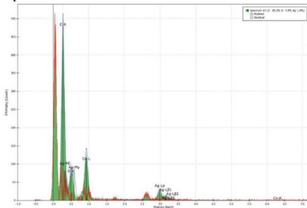
Figure 8. EDX spectrum of AgNPs. Inset the TEM micrograph of silver nanoparticles pellet solution for silver elements
