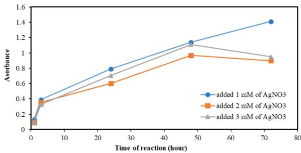
Figure 4. Time dependent-absorption for the reduction of the *Spirogyra* sp. extract with different values (1.0 mM, 2.0 mM and 3 mM) of AgNO<sub>3</sub> concentrations at the SPR peak of 488 nm
