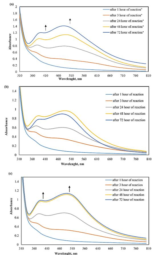
Figure 3. The reduction of the  $Ag^+$  at different concentrations by the constant amounts of aqueous *Spirogyra* sp. extract were also monitored as a function of time of reaction by UV-vis spectroscopy measurements. The spectra obtained as a function of time in the presence of 1mM (a) 2 mM (b) and 3 mM (c) of  $AgNO_3$ .
