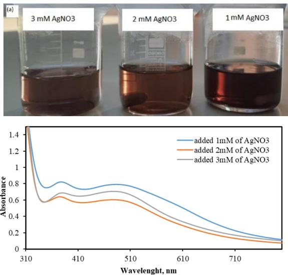
Figure 5. a) Visual appearance of the beaker containing the *Spirogyra* sp. extract and AgNO<sub>3</sub> added the *Spirogyra* sp. extract solution (1mM, 2mM and 3mM). b) UV-Vis spectra showing the effect of different conc. of AgNO<sub>3</sub> concentration on the AgNPs. The reaction time was 24 h
