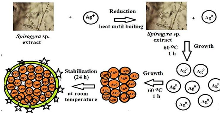
Figure 1. Schematic representation for the green biosynthesis of AgNPs from *Spirogyra* sp.
