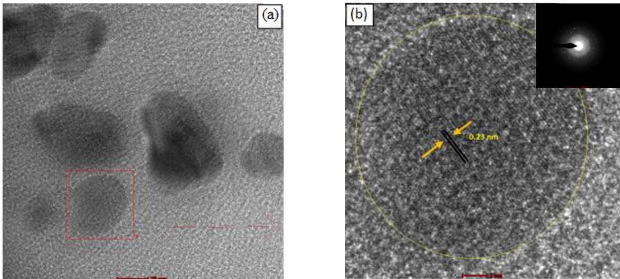
Figure 7. HRTEM images of AgNPs at 10 nm (a) and of spherically-shaped AgNPs at 2 nm which is marked in red in (a) showing fringer spacing of 0.23 nm (b). Inset in (b) is its corresponding SAED
