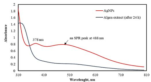
Figure 2. UV-vis spectra of the water-diluted *Spirogyra* sp. extract solution and the synthesized AgNPs solution using 1mM  $AgNO_3$  at the end of 24 h of reaction
