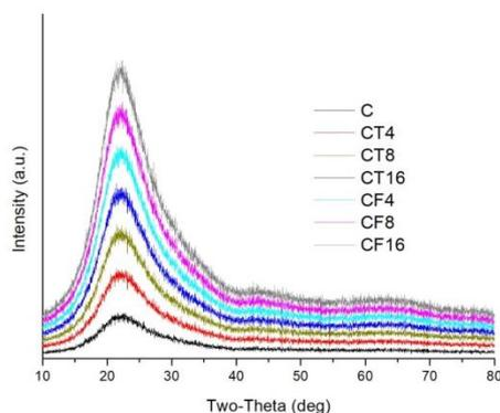
Figure 3 XRD patterns of catalysts
