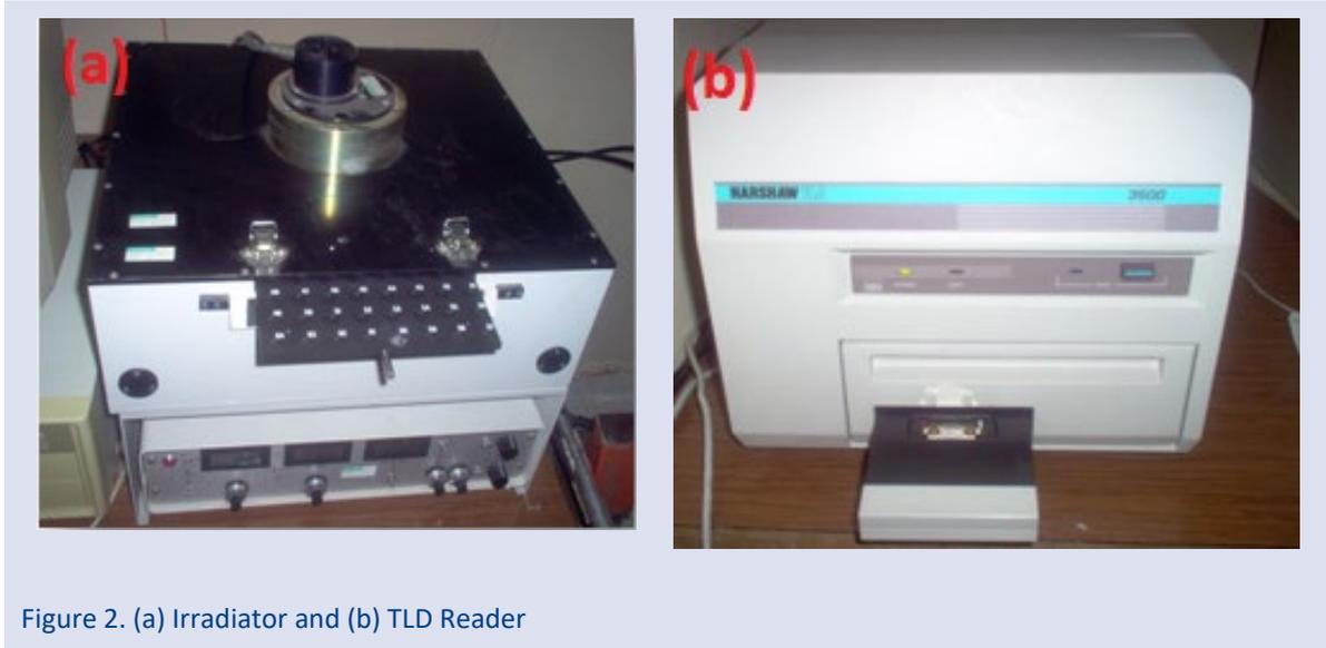
Figure 2. (a) Irradiator and (b) TLD Reader
