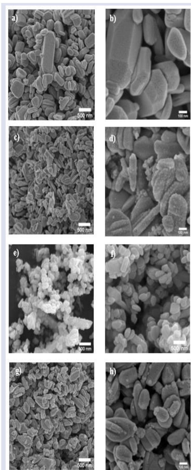
Figure 1. SEM images of nanomaterials, a-b) ZnO NPS (50K-10K), c-d) CQDs@ZnO NPs in DMF (50K-10K), e-f) C@ZnO NPs in DMSO (25K-15K), g-h) CDs@ZnO NPs (50K-10K).
