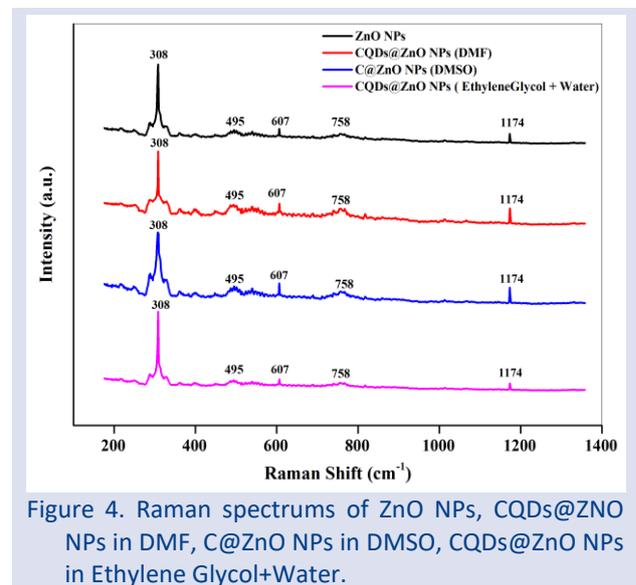
Figure 4. Raman spectrums of ZnO NPs, CQDs@ZnO NPs in DMF, C@ZnO NPs in DMSO, CQDs@ZnO NPs in Ethylene Glycol+Water.
