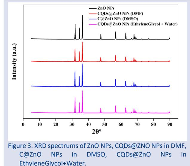
Figure 3. XRD spectrums of ZnO NPs, CQDs@ZnO NPs in DMF, C@ZnO NPs in DMSO, CQDs@ZnO NPs in EthyleneGlycol+Water.
