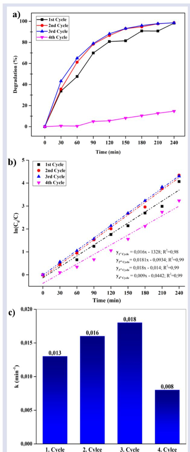
Figure 6. a) Reusability studies degradation percentage of MB concentration b)  $\ln(C_0/C)$  result of reusability studies. C) Reaction kinetic constants of each reusing reaction.
