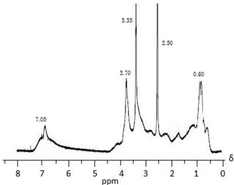
**Figure 3.** H-NMR spectrum of FN/ANE/VIBE/Stb (DMSO-d<sub>6</sub>)
