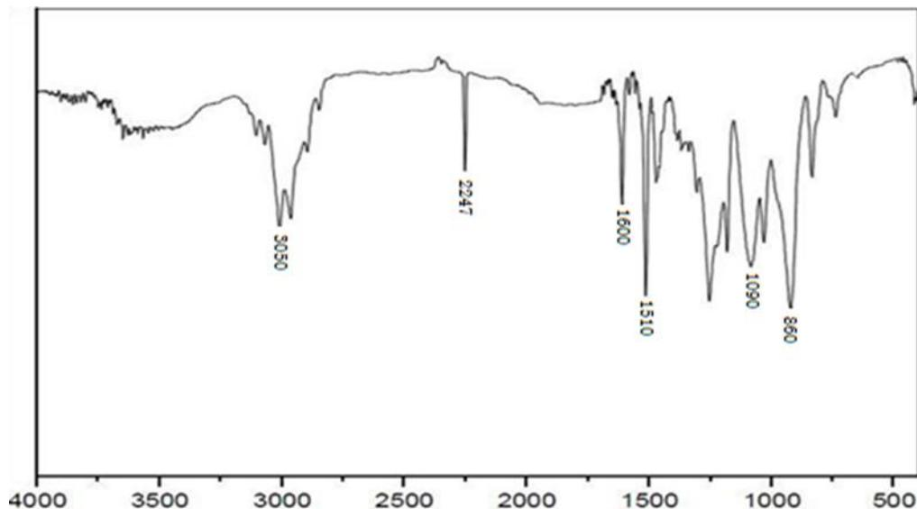
**Figure 2.** FT-IR spectrum of FN/ANE/VIBE/Stb (KBr Pellet)
