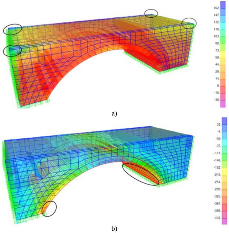
**Fig. 7.** Static analysis a) maximum tensile contour b) maximum compressive contour
