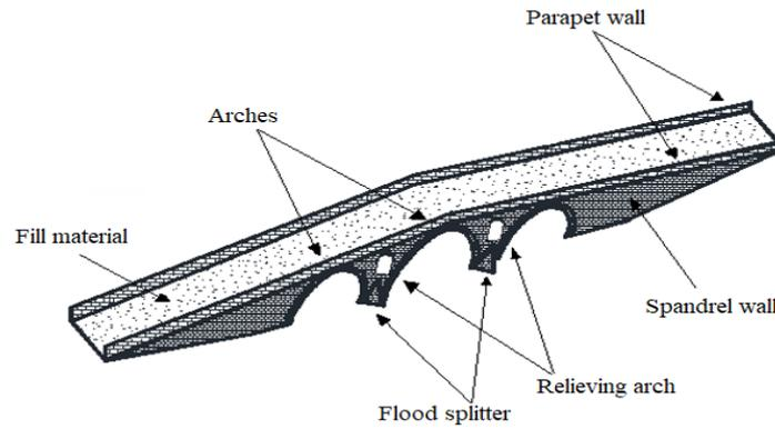
Figure 1. Typical components of masonry arch bridge
