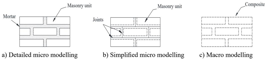
Figure 2. Modelling techniques of masonry structures [19]
