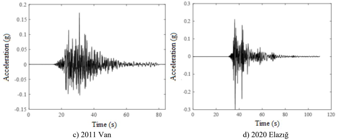
Fig. 9. East-West component of the selected earthquakes
