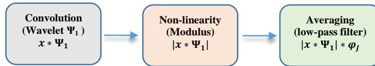
**Fig.2.** Representation of the wavelet scattering transform process with an x input.
