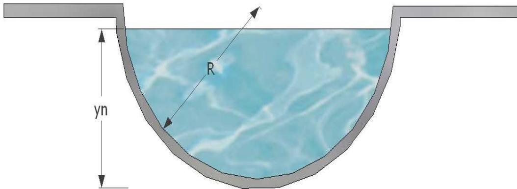
Fig. 4. Geometric dimensions of open canal with circular cross sections
