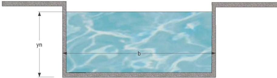
Fig. 2. Geometric dimensions of open canal with rectangular cross sections
