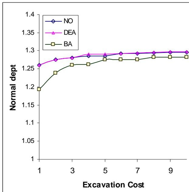
Fig. 6. Variation of optimum nondimensional side slope and normal depth of a triangular section with  $\beta_A = 0.5$
