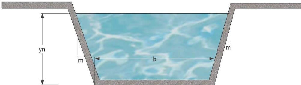
Fig. 3. Geometric dimensions of open canal with trapezoidal cross sections
