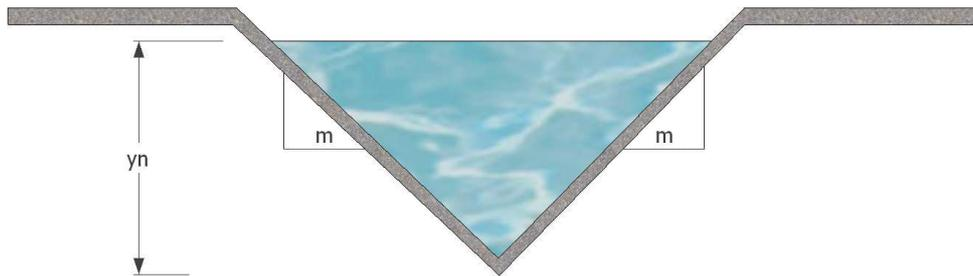
Fig. 1. Geometric dimensions of open canal with triangular cross sections
